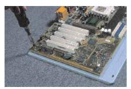
Remove the back panel from the cabinet and connect the motherboard to the panel
