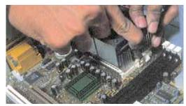
Apply a thin film of thermal paste to the heat sink
