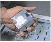
Attach the heat sink to the processor
