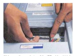
Make sure the conductor of the IDE cable which is coloured red is adjacent to the power connector
