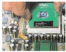
Mounting the processor the motherboard
