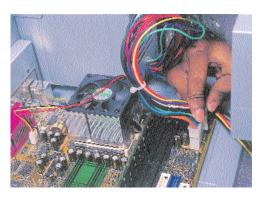
Install the power supply. Connect the main power cable to the motherboard
