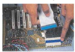
Connect the hard drive cable to the primary IDE slot
